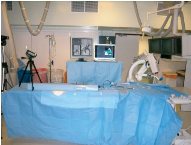
Figure 3. Set-up of the Symbionix Angiomentor Express™ simulator in the angiosuite prior to performing a patient-specific procedure rehearsal. Components include: 1, video camera (for recording of hand movements); 2, fluoroscopy monitor; 3, laptop computer; 4, mechanical interface ‘haptics’ device; 5, sheath through which endovascular tools are inserted
